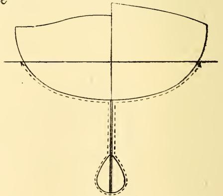
excess of draught at any point forward of that station, over the draught at that station (*see e e*, Fig. 2). For the purposes of these measurements any hollow in the fore and aft under-water profile must be treated as if filled up straight (as, *e.g.*, by the line *c d* in Fig. 1).
