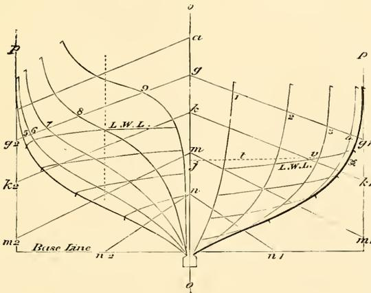
FIG. 167. BODY PLAN OF PENZANCE LUGGER.
