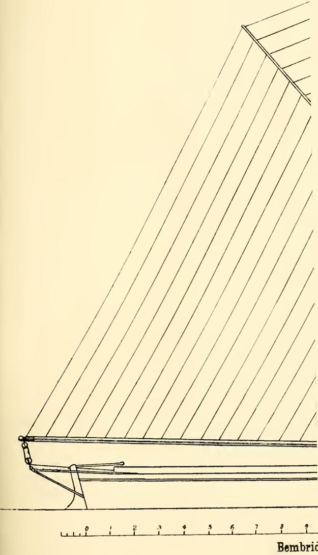
of square, so that to reef it is only necessary to turn the mast round in its step and roll up the sail; the outhaul leads through a sheave in the boom end, and is rolled round the mast the opposite way to the sail, so that if
