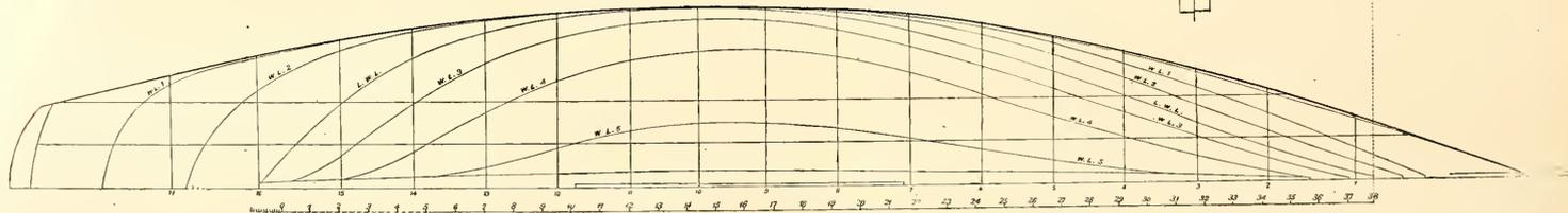
The Witch has oak frames spaced as shown, with  $\frac{1}{2}$  in. wrought iron floor-knees. Between each pair of frames is a steamed timber of American elm.
