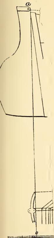
It will be seen that the sails are not laced. The boom is fitted with goose-neck or jaws to the mast, and the tack is bowsed down by a rope which leads through a block on the aft side of mast on the deck.
