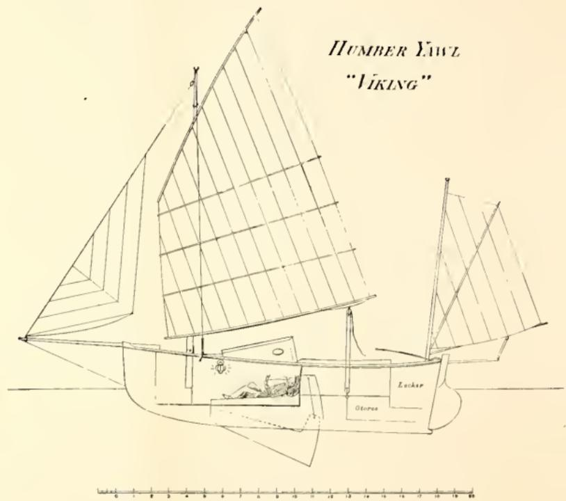
the other, is carvel built; plank,  $\frac{3}{4}$ in.; timbers, lin.  $\times$   $\frac{3}{4}$ in.; spaced  $7\frac{1}{2}$ in. Ballast, 6 cwt.
