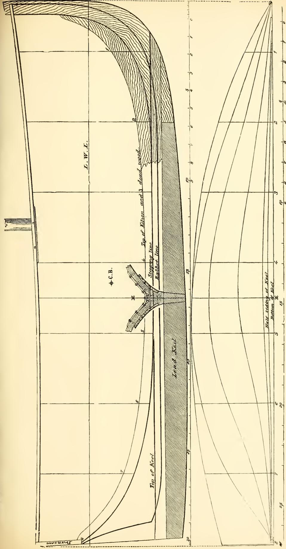
The "Gipsy," Itchen Boat, 27ft. in length. Also a Scale for a 30ft. 4in. boat on the same lines, with 9ft. 6in. boat.
