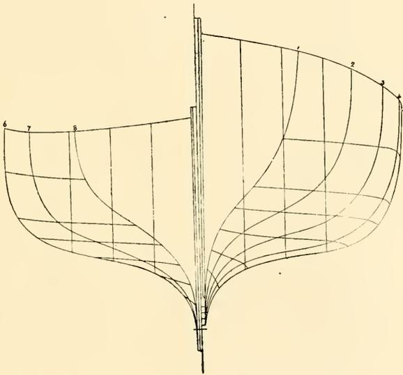
FIG. 179.—MIDSHIP SECTION OF EAST COAST SCOTCH FISHING BOAT.
