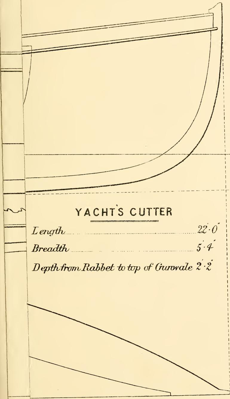
With such sails the boat, if built of the usual strength, would take about 5 cwt. of ballast. (See Plate XXVI.)
