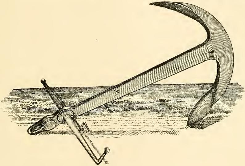
sketch (Fig. 229). The end of the cable will be fast to the wink, and as the latter is hove round the cable will be wound up. If there be two hands in the boat the cable need not be fast to the wink, but one hand can heave whilst the other holds on to the cable and coils away. A ratchet and pawl are sometimes fitted to the wink. Messrs. Pascal Atkey and Son, Cowes, manufacture a suitable ratchet windlass and also a capstan for small yachts.
