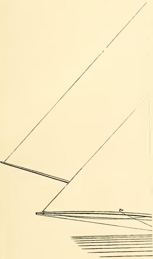
For centre board boats of the *Una* type various rigs are used, and on the *Seine* the French have brought into use an adaptation of the "sliding gunter rig." The drawing on Plate XXVII. illustrates this rig.
