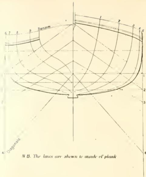
N.B. The lines are shown to inside of plank
