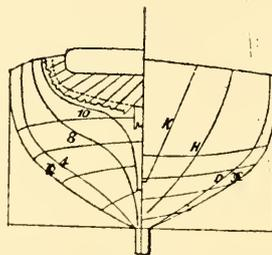
FIG. 183.—BODY PLAN OF "DIAMOND."
